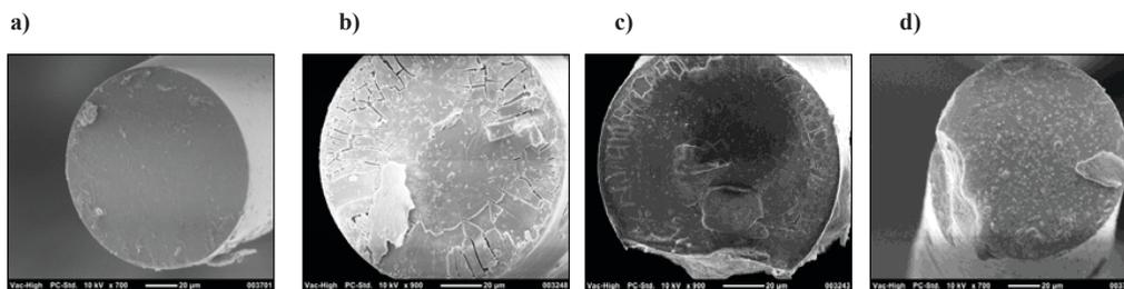
**Figure 1.** SEM imaging of optical fibers. a) Bare optical fiber. b) After 4 hours in upwards direction. c) After 4 hours in downwards direction. d) After 17 hours of hydrothermal condition in upwards direction.
