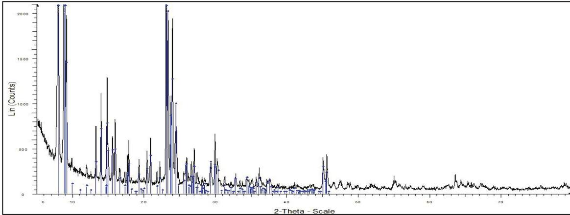
**Figure 2:** XRD result of the coating on the optical fiber end face. Typical pattern of MFI also shown (blue lines).
