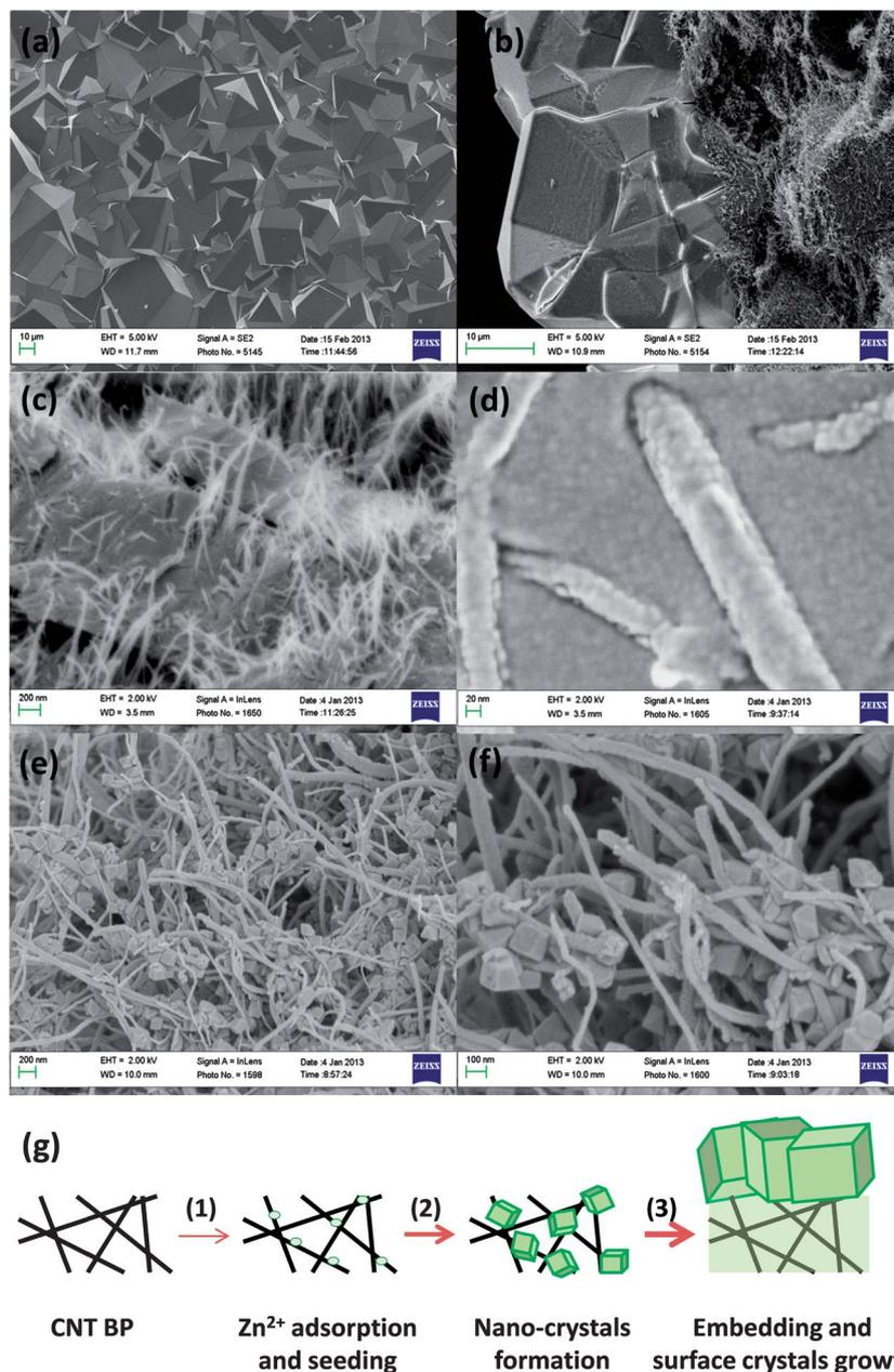
**Fig. 1** SEM of the ZIF-8–CNT BP composite membranes; (a) top surface of the ZIF-8 hybrid membrane with clear macro-sized ZIF-8 crystals; (b) cross section view of ZIF-8 hybrid membrane; (c) embedded coarse CNTs within the ZIF-8 matrix; (d) view of a ZIF-8–CNT interface; (e) and (f) evidence of the formation of ZIF-8 nano-crystals on the CNTs during the early stage of ZIF-8 growth.
