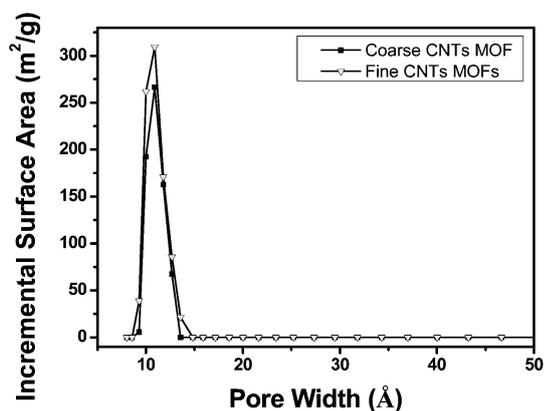
**Fig. 4** Pore size distribution calculated from the BJH-BET model from N<sub>2</sub> adsorption for the two types of samples. Fine CNTs were shown to lead to slightly narrower pore size distribution, but no major changes were found confirming the homogeneity of the two structures.
